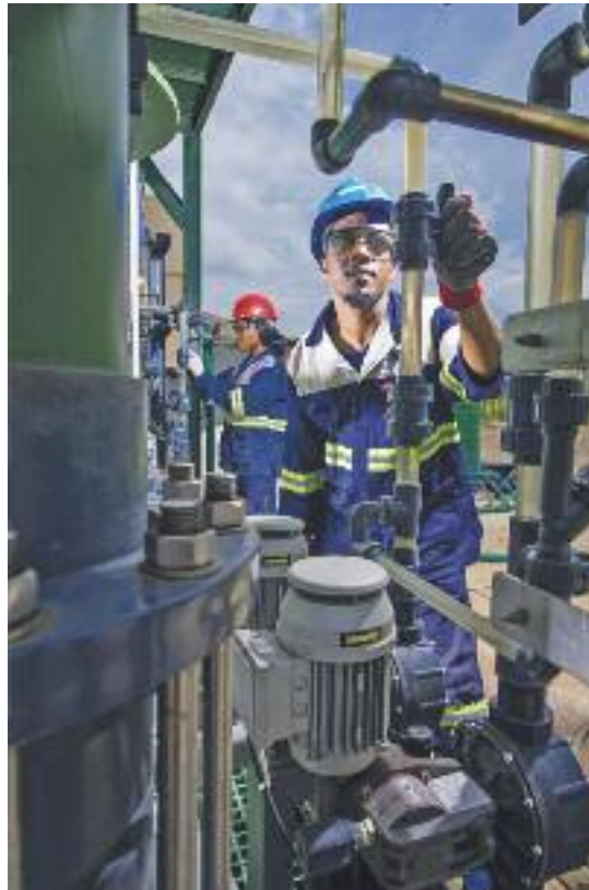
A single-stage Clean TeQ CIF module can be used for a range of treatment applications. Multotec focuses on the Dual-stage Iconic Desalination (DeSALx) process in South Africa, to produce water with low total dissolved salts (TDS) and a neutral pH
